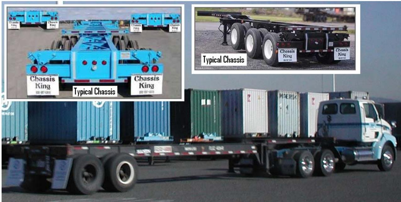
The I-Beam chassis is different from a typical flatbed chassis shown in Figure 8. A flatbed chassis is not a container chassis used to transport Port cargo and thus a tractor with a flatbed chassis was recorded based on the number of axles of the truck, but was not counted as a Port-related vehicle.
