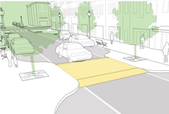
Vertical Speed Control Elements Speed Humps, Tables, Cushions
